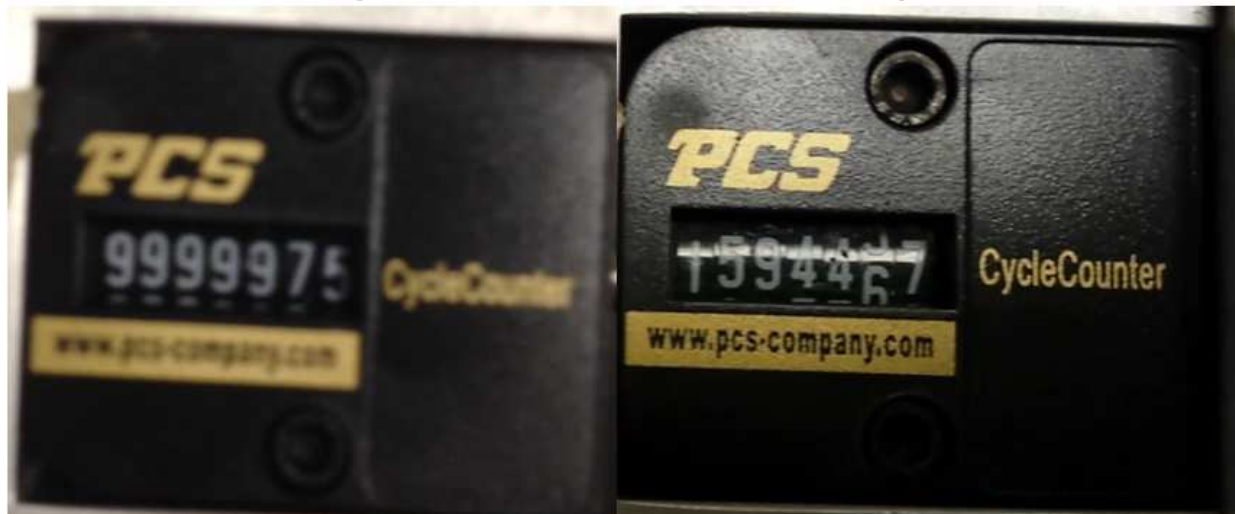
Figure 6 – Counter 4 before and after testing.
