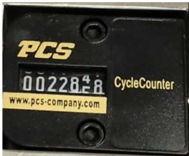
Figure 13 – Counter 8 at failure.
