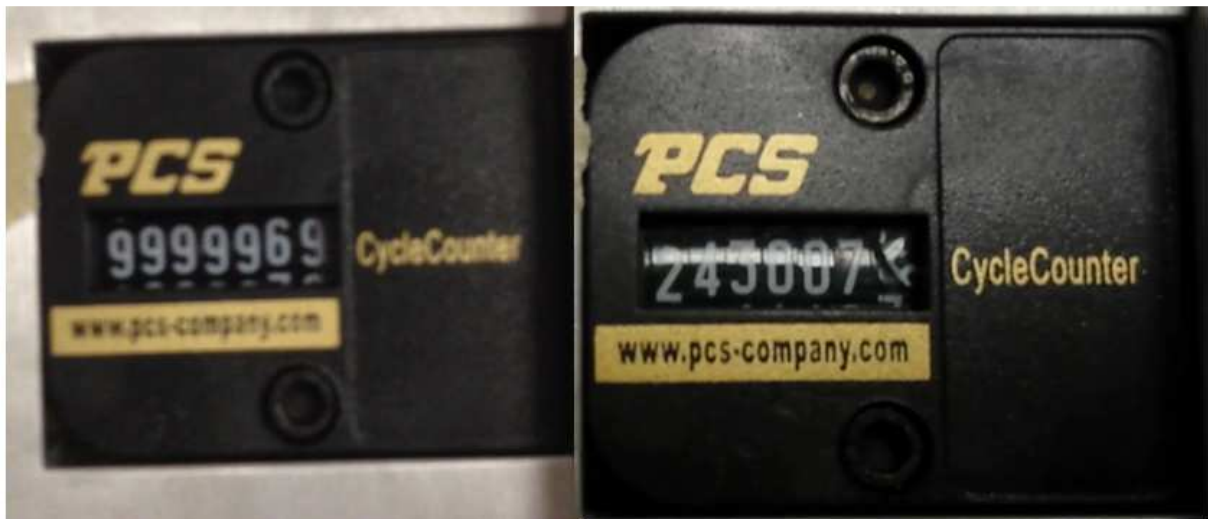
Figure 3 – Counter 2 before and after testing.
