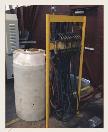
Aalbers used this homemade water testing system for many years, but it was messy and labor-intensive, and lacked any means for securely recording and archiving waterline analyses. And because it was bolted to the floor, molds had to be moved and staged near the apparatus anytime testing was done.
