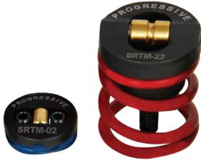
Progressive's SRT® Series Slide Retainers reliably hold from 2 to 80 pounds (1 to 36 kgs) each. This slide retention design now features color-coded springs to indicate force rating. This compact design allows for installation in a mould base or wear plates.
