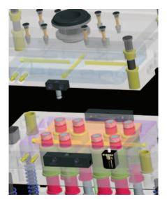
New products are now available for zero clearance mold alignment, grease-free parting line sequence control, and standardized runner puller pins and bushings for three plate runners.
