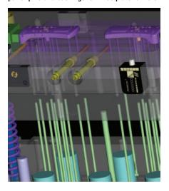
New tooling can now benefit from inlet cascades to route cooling lines into tight spaces.
