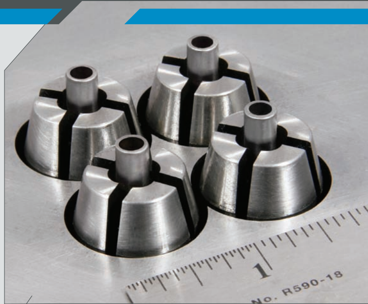
Close cavity spacing can allow the use of a single, multi-tip nozzle, reducing the costs and variables introduced by a manifold system required in a tool with side actions.
